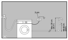
Make sure that it is designed in such a way, that the end of the drain hose cannot be covered with water. The drain hose may be extended to a maximum of 4 metres. An additional drain hose and joining piece is available from your local Service Force Centre. The joining piece must have an internal diameter of 18mm.
